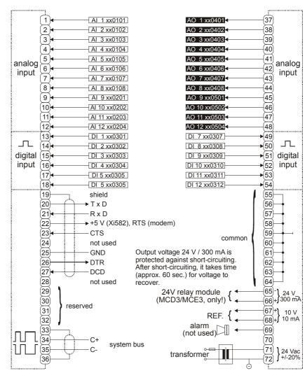
**NOTE:** Terminals 65 and 66 provide a pulsed 24 Vdc output, and can only be used to connect relay modules MCD3/MCE3. Do not connect relays to these terminals!
